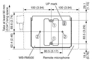
1 Hole for the switch box (Also used for direct wall mounting)
